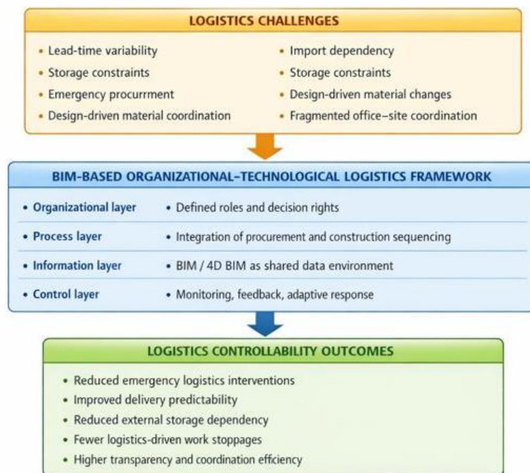
Fig. Conceptual representation of BIM-based logistics integration and its impact on construction process controllability
